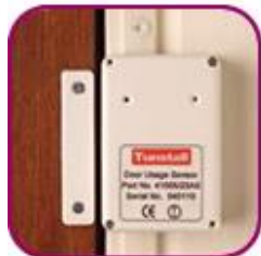
Door exit sensor
